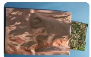
Packaging can outgas and contaminate the part
