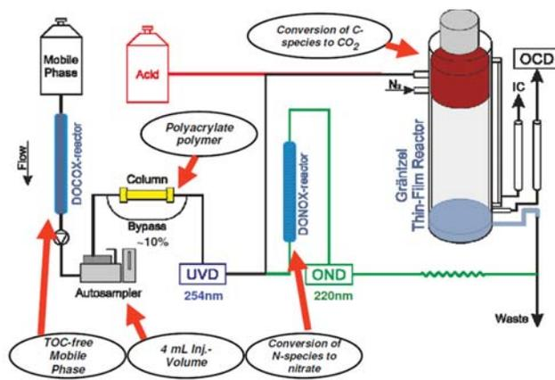
Figure 2. LC-OCD schematic diagram
