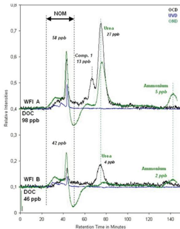
Figure 1. Analysis of water for injection in pharmaceutical applications
