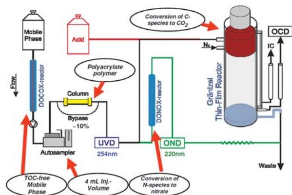
Figure 3. LC-OCD schematic diagram
