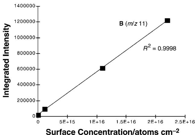
Fig. 3 Calibration plot for boron implant constructed from wafer standards.
