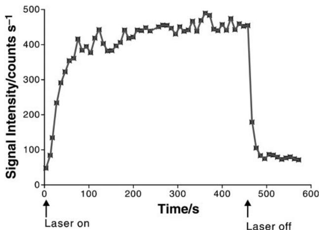
Fig. 2 Time-resolved <sup>11</sup>B<sup>+</sup> signal profile obtained with a boron-doped Si wafer.
