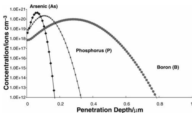
Fig. 1 Simulated concentration versus penetration depth.
