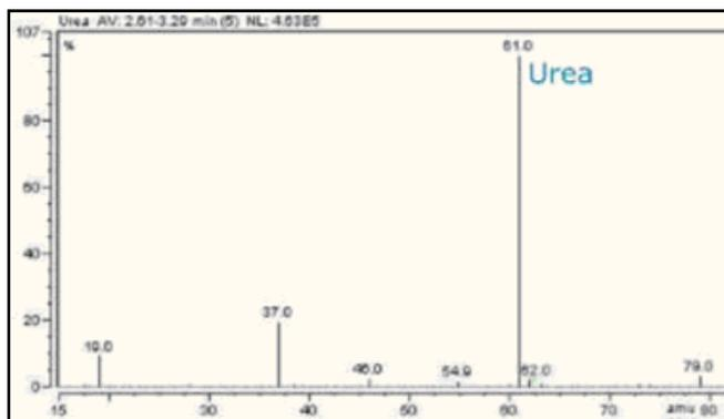
Using this IC-MS technique Balazs has detected urea at concentrations down to 0.6 ppb, and can provide analyses on feed city water, process water used in the fab, as well as reclaim water for DIW and process engineers. DIW purities and concerns evolve, so does our analytical arsenal.
