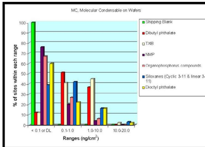
Fig. 1 Organic Contamination on Wafers
